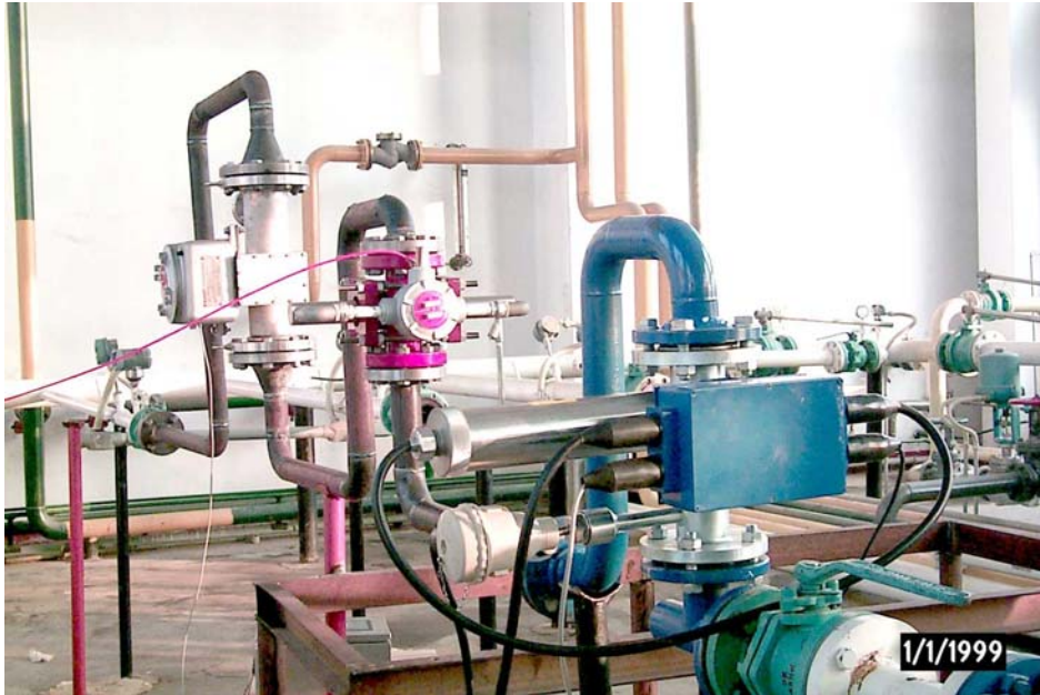
Figure 4. Picture showing the three meters connected in series during the test (Date on the picture is incorrect because of wrong date setup in the camera)
